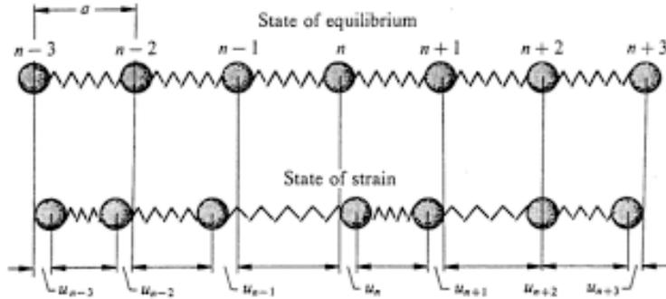
**Fig 4 chain of one-dimensional harmonic oscillators**
